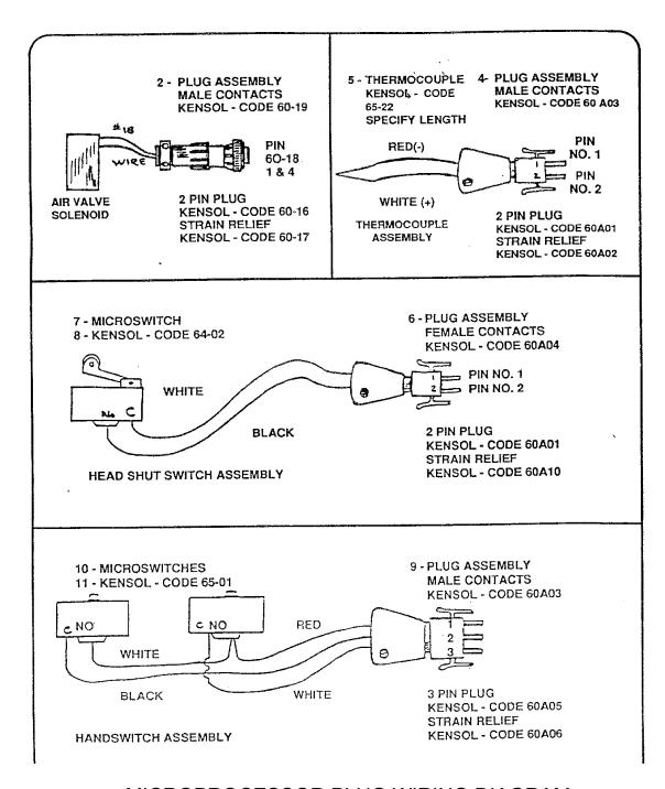
MICROPROCESSOR PLUG WIRING DIAGRAM
