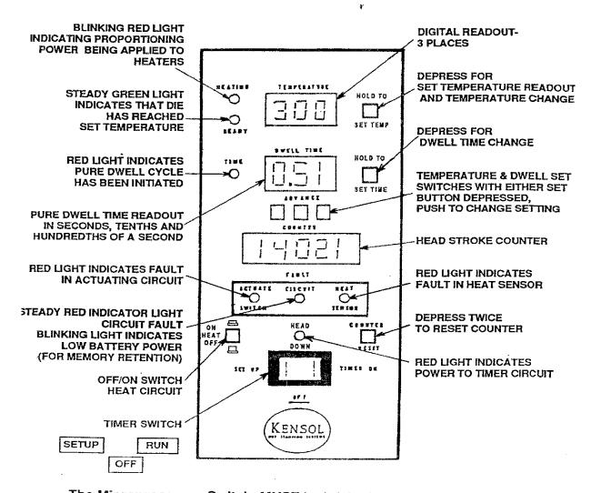
The Microprocessor Switch <u>MUST</u> be left in the "<u>OFF</u>" (Mid Position) when <u>Disconnecting</u> or <u>Connecting</u> the Electricity or <u>Removing</u> Plug
